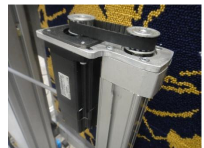
Y drive and enclosed actuator (guard removed)
