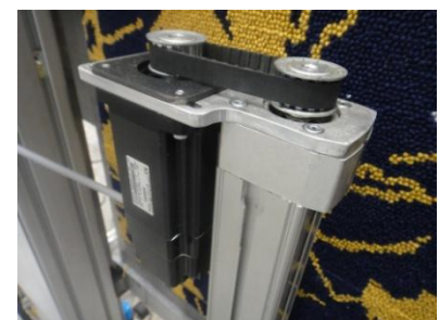
Y drive and enclosed actuator (guard removed)
