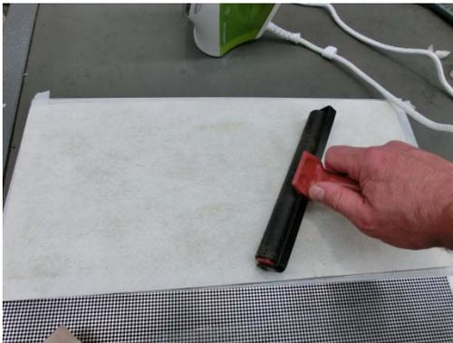
The Roller is used to smooth and force the hotmelt into the back of the tufts
