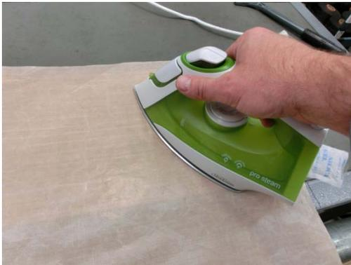
A conventional iron is used to heat the holt melt evenly across the entire sample. If necessary, heat a section of hotmelt at a time.
