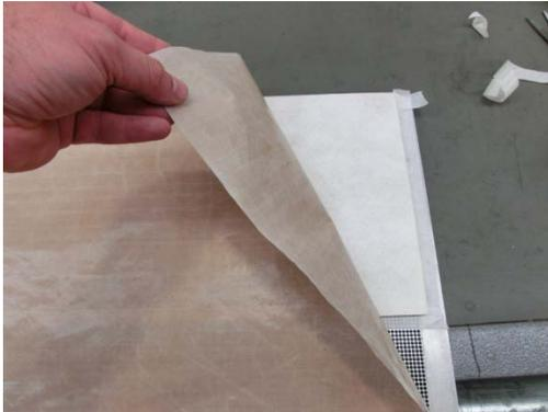
The teflon sheet is laid over the back of the hotmelt
