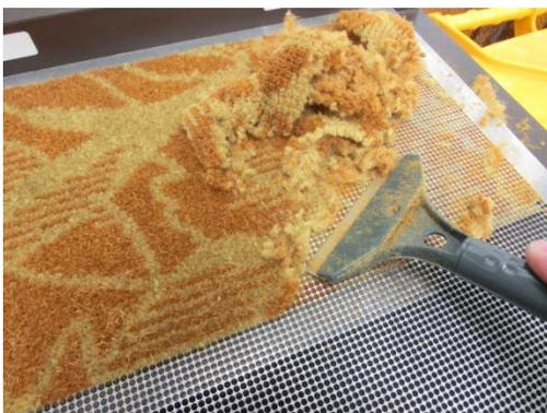
The pegboard is turned over, the scraper is used to shear the cut side of the sample level with the surface of the pegboard.
