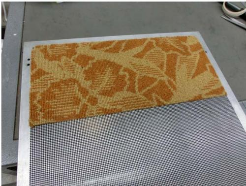
A Kibby sample is produced on the Kibby machine. In this instance, the sample is half the pegboard full size.
