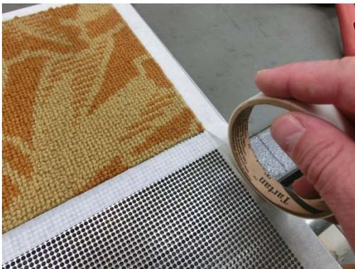
The Pegboard is protected from Hot Melt Adhesive with masking tape.
