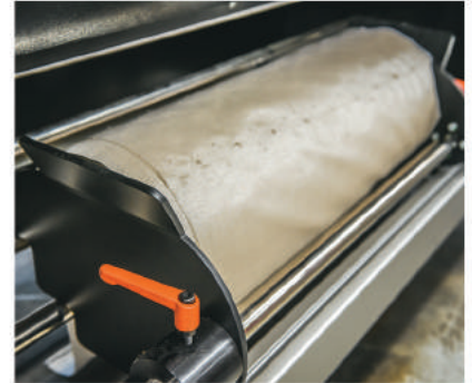
Primary backing roll with quick change side guides
